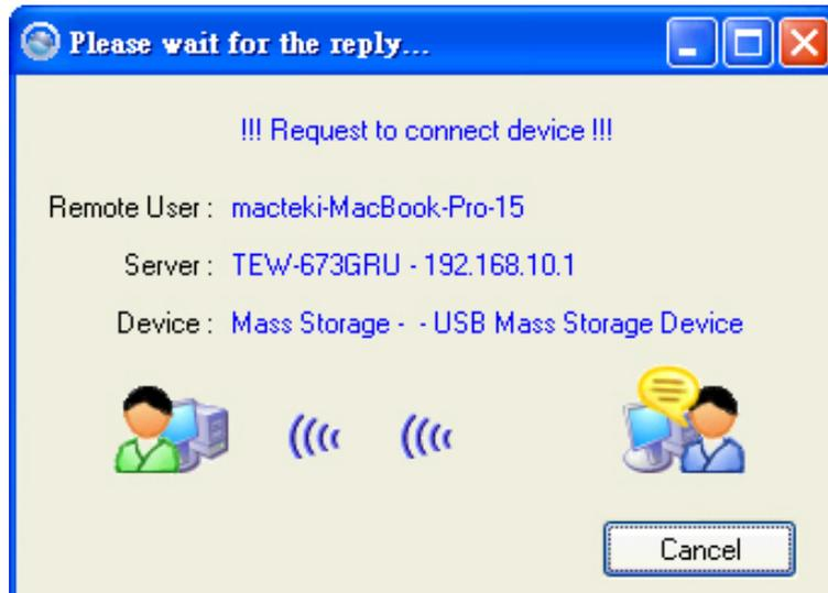
Note: Only a single user can establish connection to a USB device. Once the “Request to Connect” is approved, the connection to the USB device will automatically transfer to the requested user.
