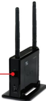
4. Connect a CAT-5 cable from the TEW-638PAP's **LAN** port to the TPE-111GI's **POE OUT** port
