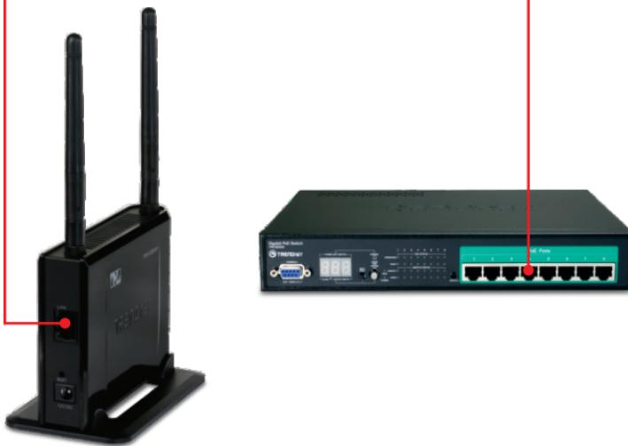
2. Verify that the wireless, LAN, and power LEDs are on.
