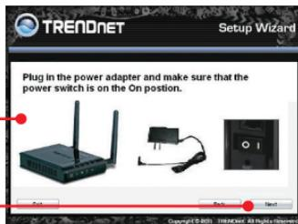
7. Connect the Power Adapter to the Access Point and then to a power outlet. Verify that the power switch is set to the on position (EU version only). Then click **Next**.
