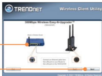
4. Connect the AC Power Adapter to the Access Point and then to a power outlet and then click **Next**.
