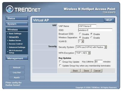
Figure 18: WPA and WPA2 with Radius Wireless Security Screen
