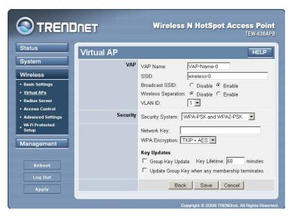
Figure 15: WPA-PSK and WPA2-PSK Wireless Security Screen
