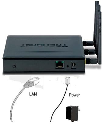
Figure 4: Installation Diagram
