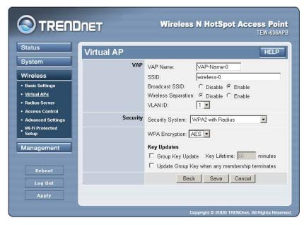
Figure 17: WPA2 with Radius Wireless Security Screen
