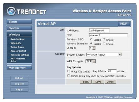
Figure 16: WPA with Radius Wireless Security Screen
