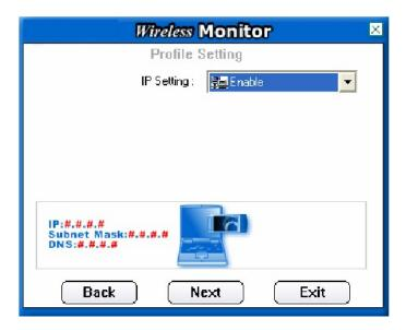
**Step 7.** Enable "**DHCP**" and click "**Complete**" if you are using a dynamic IP address. If you are using a static IP address, disable "**DHCP**" and manually enter the desired IP address, subnet mask, default gateway and DNS server addresses then click "**Complete**".
