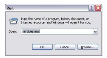
**Step 2.** This will open the services window. Double click on the **Wireless zero configuration** service.
