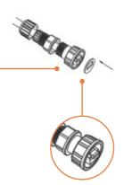
**10.** Connect the clamp ring and seating nut to the **PoE** port on the rear of the TEW-455APBO.
