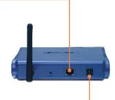
2. Connect the AC Power Adapter to the Access Point and then to a power outlet.
