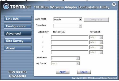
Encryption: 4 options are available: Shared Key, Auto, WPA/WPA2 and WPA-PSK/WPA2-PSK. Select Shared Key or Auto for WEP data encryption feature. Shared Key – the sender and receiver shares the common key for data communication, and the key is used for extended length of time.
