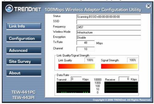
**Status:** Shows the BSSID associated, which can be used to identify the wireless network.
