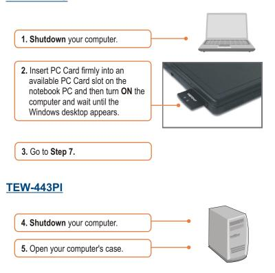
6. Insert PCI Card firmly into an available PCI Card slot on the desktop PC, attach the included antenna, and then turn ON the computer and wait until the Windows desktop appears.
