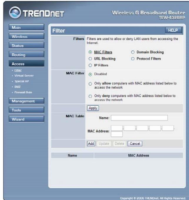
**MAC Filter:** Enables you to allow or deny Internet access to users within the LAN based upon the MAC address of their network interface. Click the radio button next to Disabled to disable the MAC filter.
