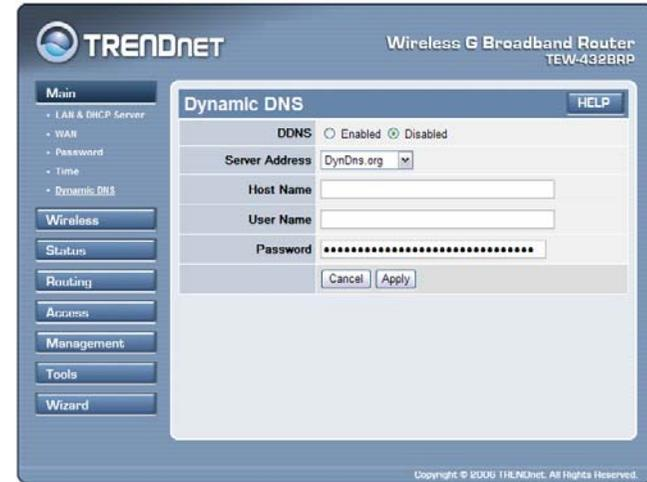
The screenshot shows the 'Dynamic DNS' configuration page for a Trendnet Wireless G Broadband Router (TEW-432BRP). The page includes a sidebar with navigation options: Main, LAN & DHCP Server, WAN, Password, Time, Dynamic DNS, Wireless, Status, Routing, Access, Management, Tools, and Wizard. The main content area is titled 'Dynamic DNS' and contains the following fields and controls:
