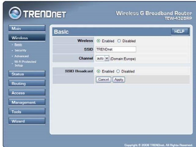
**Enable/Disable:** Enables or disables wireless LAN via the WLAN Router.
