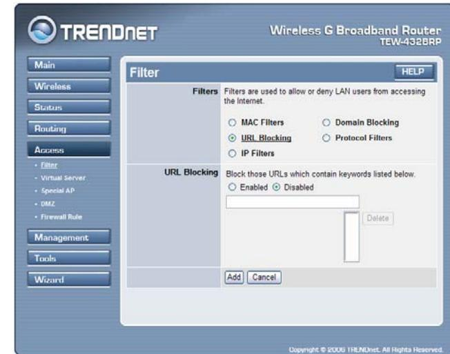
**Enable / Disable:** Enable or Disable the URL blocking function of the WLAN Router.
