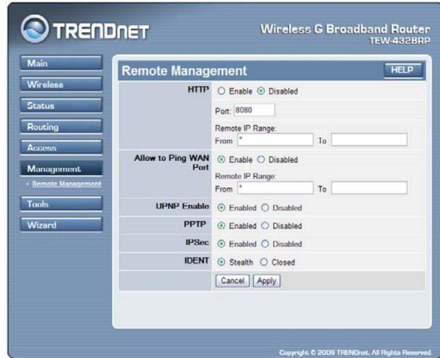
**HTTP:** Enables users to set up HTTP access for remote management.
