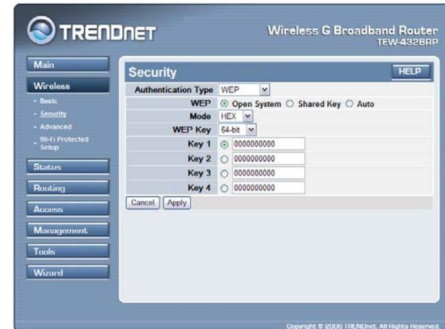
**WEP:** Open System and Shared Key requires the user to set a WEP key to exchange data with other wireless clients that have the same WEP key..
