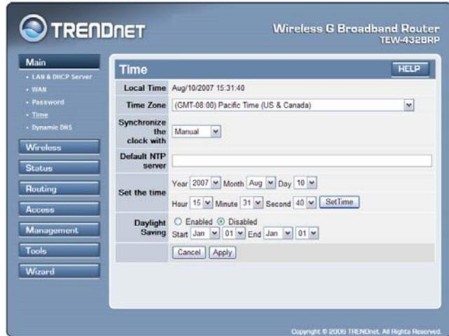
The screenshot shows the 'Time' configuration page for a Trendnet Wireless G Broadband Router (TEW-432BRP). The page includes a sidebar with navigation options: Main, LAN & DHCP Server, WAN, Password, Time, Dynamic DNS, Wireless, Status, Routing, Access, Management, Tools, and Wizard. The main content area is titled 'Time' and contains the following fields and controls:
