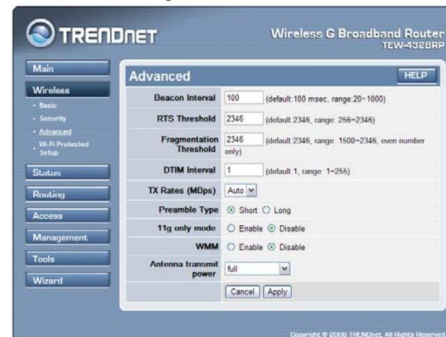
**Beacon Interval:** Type the beacon interval in the text box. User can specify a value from 20 to 1000. The default beacon interval is 100.
