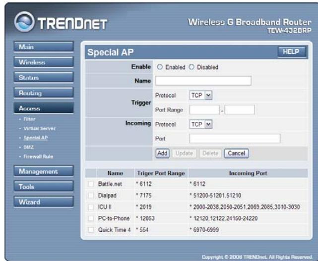
**Enable:** Click to enable or disable the application profile. When enabled, users will be able to connect to the application via the WLAN Router’s WAN connection. Click “Disabled” on a profile to prevent users from accessing the application on the WAN connection.
