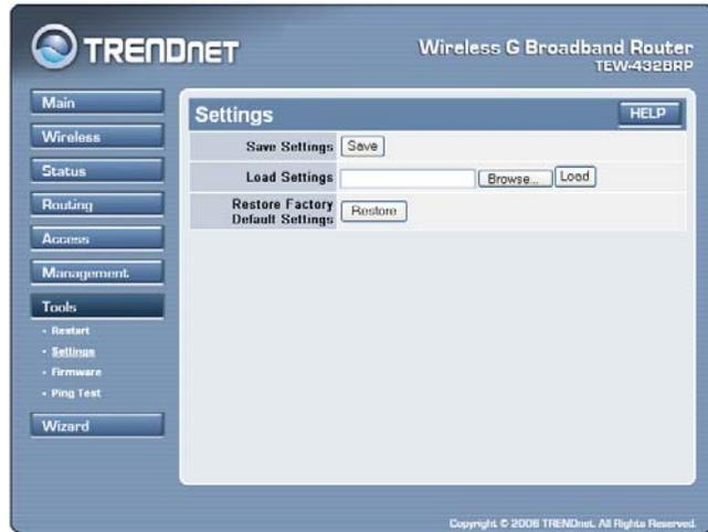
**Save Settings:** Click “Save” to save the current configuration as a profile that can load when necessary.
