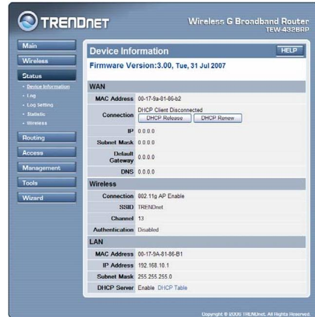
**Firmware Version:** Displays the latest build of the WLAN Router firmware interface. After updating the firmware in Tools - Firmware, check this to ensure that the firmware was successfully updated.
