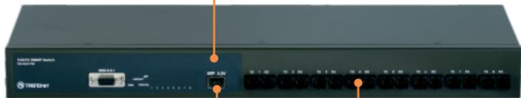
3. Connect a Fiber cable to one of the ports on the switch and to a fiber connection on your network.
