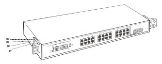
Figure 2. Combine the Switch with the provided screws
