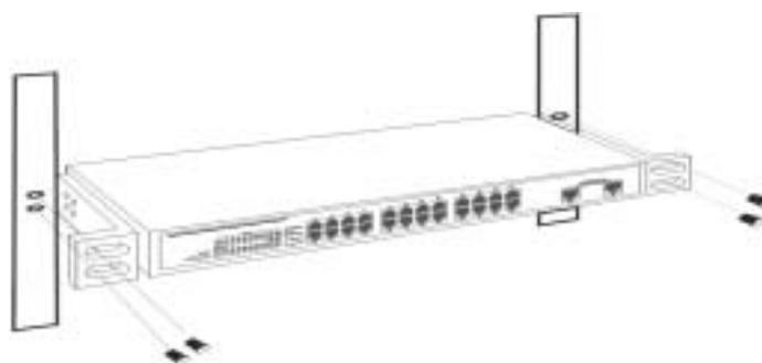
Figure 2. Mount the Switch in the rack
