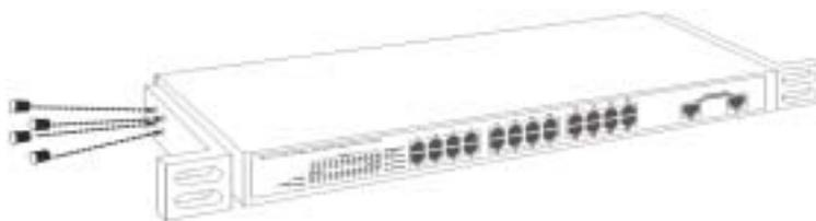
Figure 1. Combine the Switch with the provided screws
