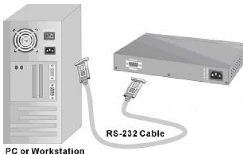
Figure 4-1. Connecting the TE100-S810Fi to a terminal via RS-232 cable
