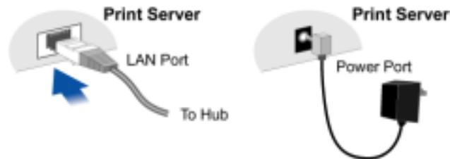
4. Connect the supplied Power Adapter, power up both the Printer and Print Server and check the Printer Server LEDs:
