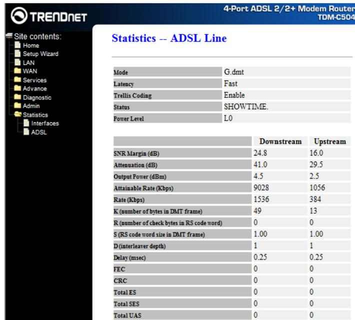
The screenshot shows the TrendNet web interface for a 4-Port ADSL 2/2+ Modem Router (TDM-C504). The page is titled "Statistics -- ADSL Line". A sidebar on the left shows a navigation menu with "Statistics" expanded to "ADSL". The main content area contains a table of ADSL line statistics.
