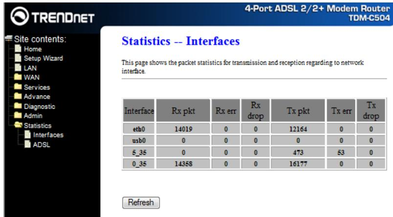
The screenshot shows the TrendNet web interface for a 4-Port ADSL 2/2+ Modem Router (TDM-C504). The page is titled "Statistics -- Interfaces". A sidebar on the left shows a navigation menu with "Statistics" expanded to "Interfaces". The main content area contains a table of network interface statistics and a "Refresh" button.
