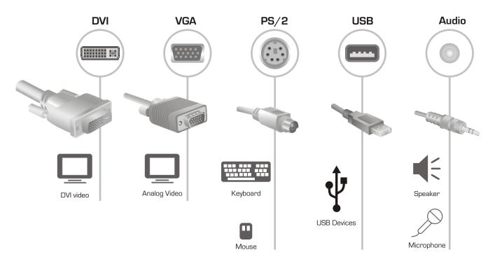
**Console Connection Interface** is generally located on the front of the KVM switch. Your common Console Interface includes two Personal System/2 (PS/2) ports for keyboard and mouse connectivity, and one Video port for computer monitor connectivity. The Console Interfaces are used to connect the primary keyboard, video and mouse for control over multiple workstations.
