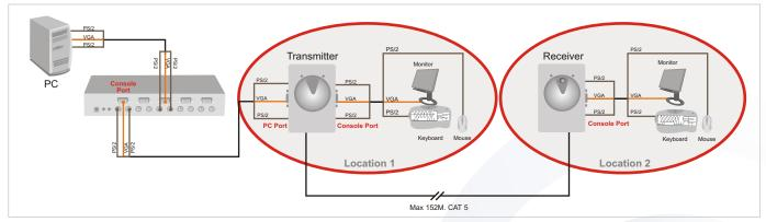
**KVM Extenders** are used when a PC is too far away from the keyboard, video and mouse peripherals or a KVM switch. Using standard KVM cables doesn't always suffice because of signal loss characteristics, which can cause fuzzy images and attenuated communication. KVM Extenders work in a simple yet effective manner by utilizing standard Category 5 Ethernet Cable to complete the remote connections from your PC to your KVM devices.
