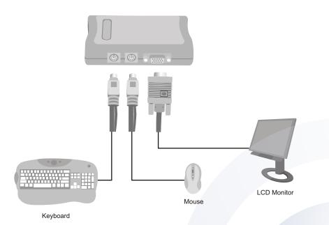
Depending on the number of ports of the selected KVM switch, you can control from 2 to 16 computers. Other enterprise KVM switches allow you to combine or "stack" KVM switches together to control from 128 to 256 computers. There are also audio-rich KVM solutions that offer digital playback and recording, and video-enhanced KVM switches that display crisp, digital images.
