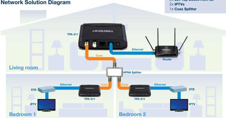
This diagram illustrates the installation of TPA-311 adapters to create a fast Ethernet connection using a home's existing coaxial cabling for IPTV streaming.
