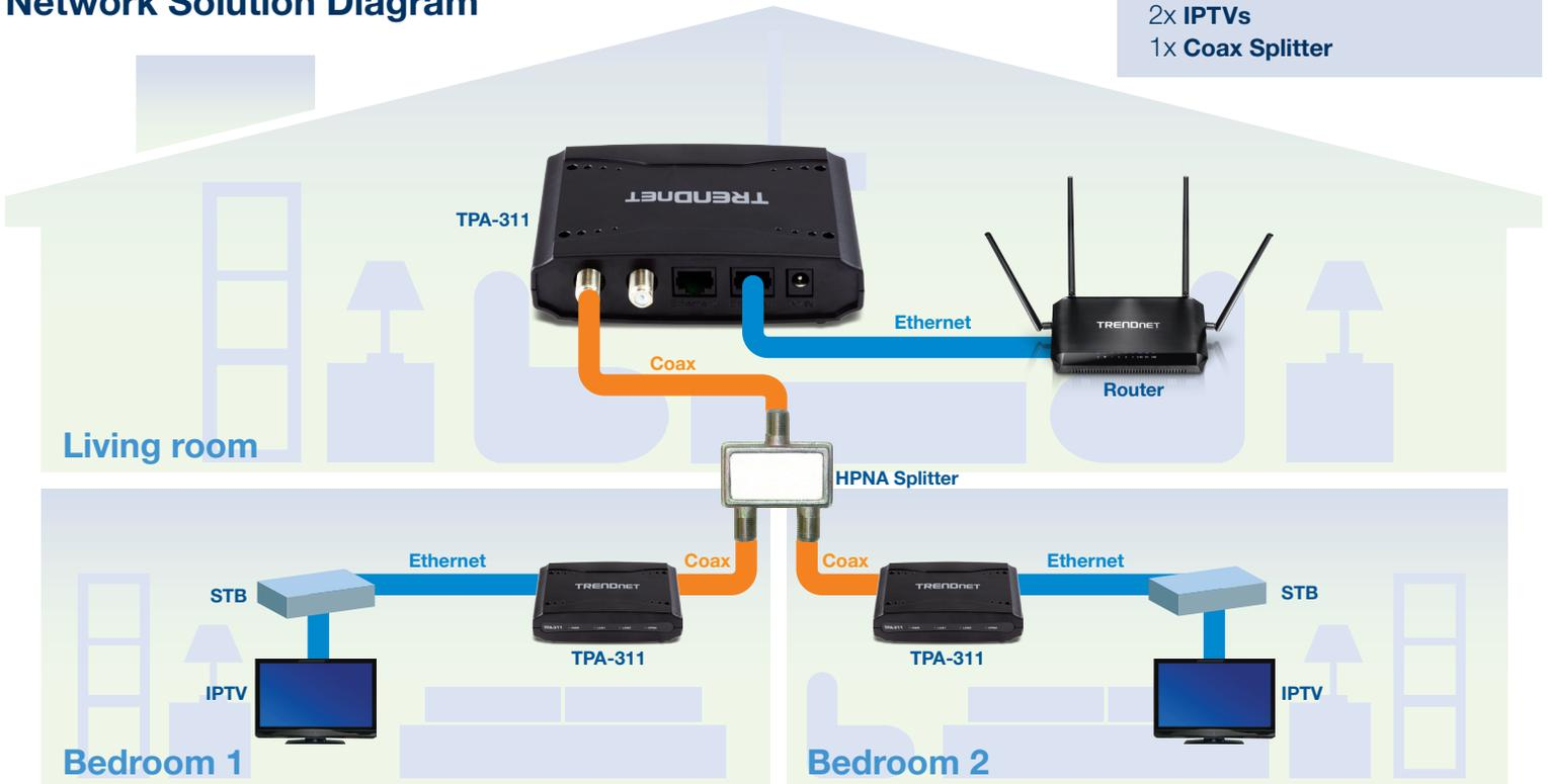
This diagram illustrates the installation of TPA-311 adapters to create a fast Ethernet connection using a home's existing coaxial cabling for IPTV streaming.
