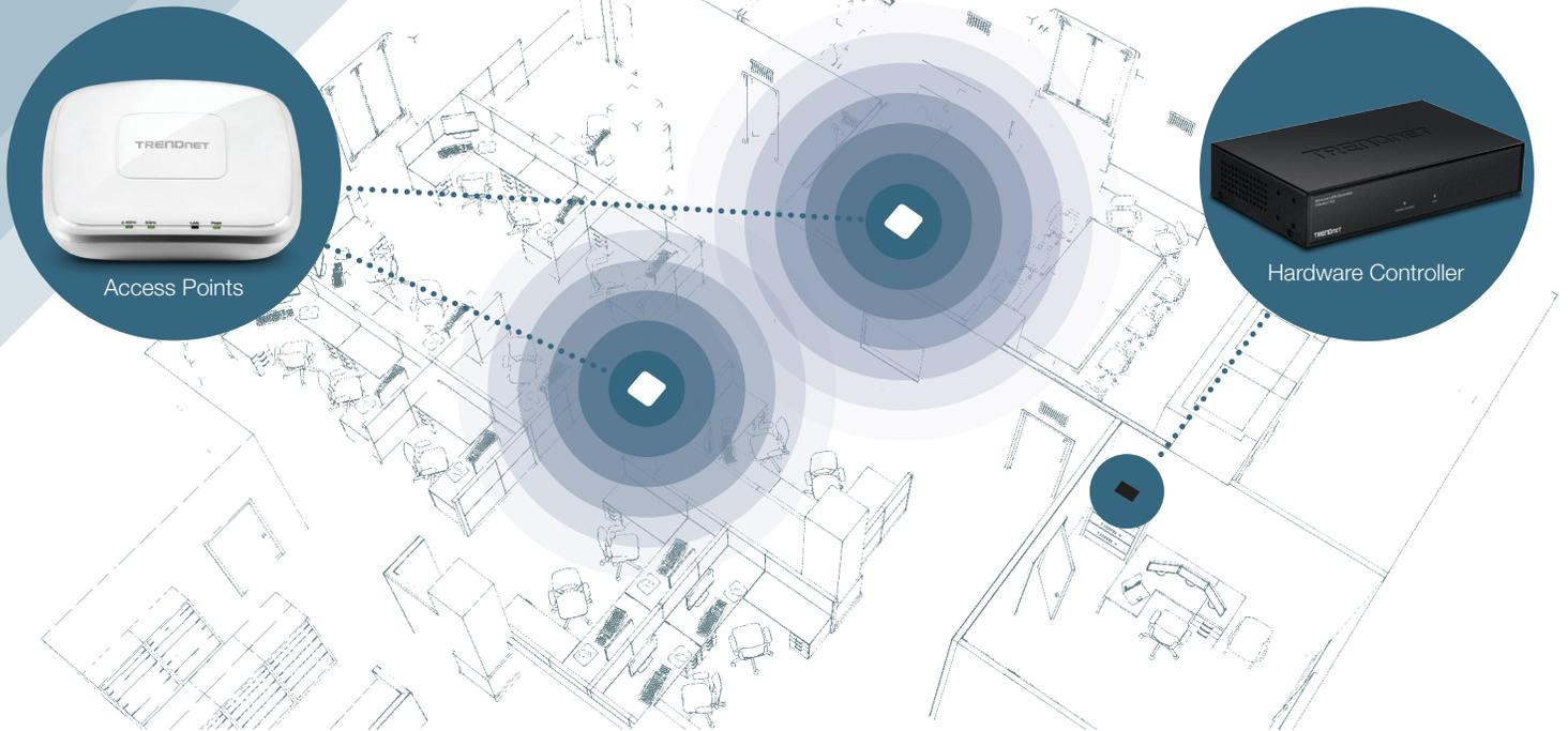
Wireless controllers provide two primary functions, centralized AP management and seamless roaming capabilities.
