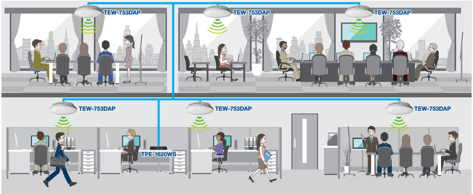
This diagram demonstrates the strategic positioning of the TRENDnet access points and web smart switch to create a roaming wireless network solution. Please note that the diagram is not to scale.
