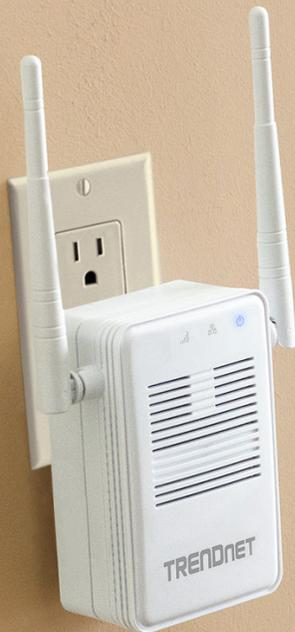
When a wireless signal just needs a little boost, a wireless repeater (or wireless extender) can get the job done. Wireless speeds have gotten much better, but the range can still be an issue especially in larger homes.
